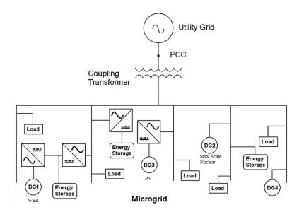
Figure 2.1: Microgrid Architecture with Mixed Energy Sources
