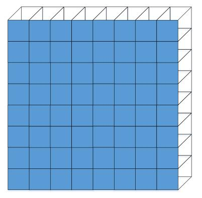
Array Assembly 65.024 cm x 65.024 cm (<.5 m<sup>2</sup>) 7 kW Radiated Power @~95 GHz (8x8 Array of 100 W+ modules)
